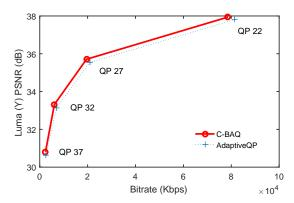
in comparison with AdaptiveQP on the 4:4:4 10-bit test sequence *ParkScene* (using the Main\_444\_10\_Intra RExt profile including the All Intra encoding configurations).
