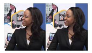
**Figure 3:** Comparison of an intra-predicted frame from the *KristenAndSara* 4:2:0 sequence at QP 37 (All Intra): (a) coded with C-BAQ — 5580.99 Kbps, (b) coded with AdaptiveQP — 5998.07 Kbps.
