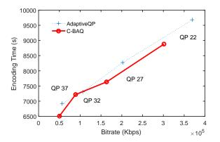
**Figure 9:** Encoding time improvements attained by the proposed C-BAQ technique compared with AdaptiveQP on the 4:4:4 8-bit test sequence *PeopleOnStreet* (using the Main\_444\_Intra RExt profile including the All Intra configurations).
