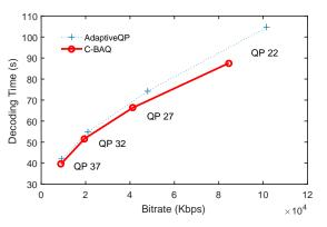
**Figure 10:** Decoding time improvements attained by the proposed C-BAQ technique compared with AdaptiveQP on the 4:2:2 10-bit test sequence *ParkScene* (using the Main\_422\_10\_Intra RExt profile including the All Intra configurations).
